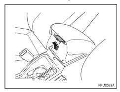
Your vehicle has a front armrest storage area. To open the storage area, pull up on the lift lever and raise the lid. To close the storage area, lower the lid and push it down until it latches securely.
